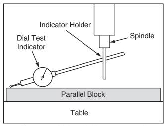
Figure 70. Dial test indicator mounted.
